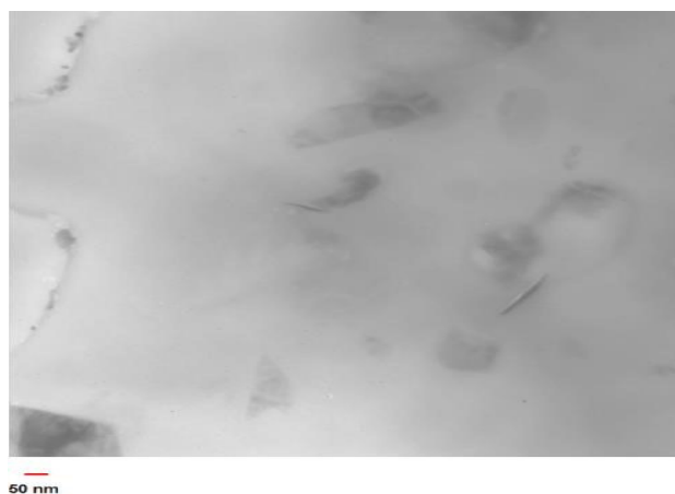
Figure 1. TEM image of the exfoliated MoS_2 .
